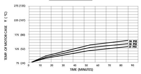
THIS GRAPH IS FOR USE AS A DESIGN GUIDE. IT IS BASED ON RUNNING CONTINUOUSLY WITH AN AMBIENT TEMPERATURE OF 70° F IN STILL AIR. THE THERMAL BREAKER WILL OPEN WHEN THE CASE TEMPERATURE REACHES 280° F.
