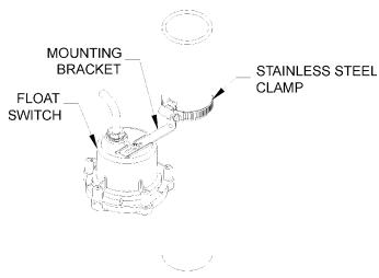
The vertical diaphragm switch provides automatic control of a pump in water and sewage effluent applications. The design allows it to operate in applications with limited space, such as small sump chambers. The VDS features models with either a 6" or 10" pumping range.
