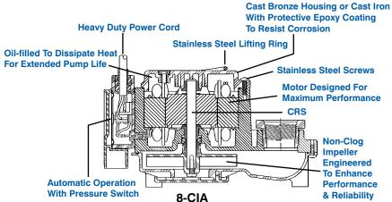
For residential and light commercial use, the Model 8 Series sump pumps provide efficient and reliable service. For extended or continuous use in moving large volumes of water, these pumps feature a 1-1/2" discharge with a maximum head of 22.9', a polycarbonate cover and a polypropylene volute/base. A choice of manual or automatic versions provides user with the right pump for their needs.
