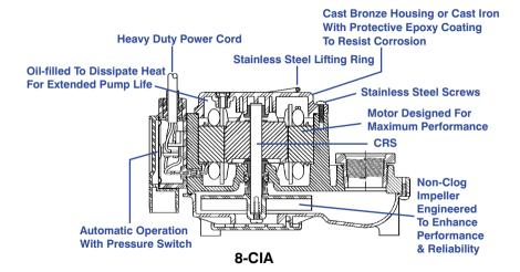
For residential and light commercial use, the Model 8 Series sump pumps provide efficient and reliable service. For
