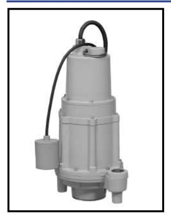
The "Magnum™" Grinder Pumps Series have an exclusive cutter assembly that cuts sewage and stringy materials into tiny particles, eliminating roping and clogging that may occur in other pumps, producing a fine slurry that passes easily through the system. Compared to standard sewage pumps, this allows use of smaller diameter discharge pipes, smaller pumps and less electricity, reducing installation and operating costs.
