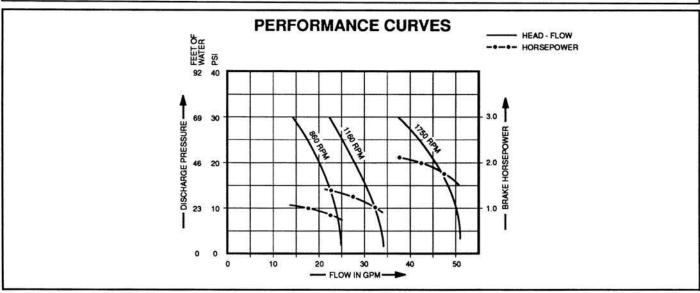
NOTE: Curve shows approximate head-flow for new pumps with neoprene impeller pumping water. Capacities should be reduced approximately 10% for nitrile, viton and EPDM impellers.
