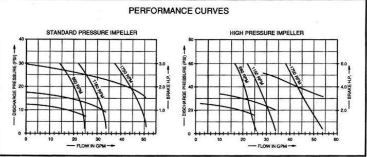
NOTE: Curves show approximate head flow for new pumps with neoprene impeller pumping water.
