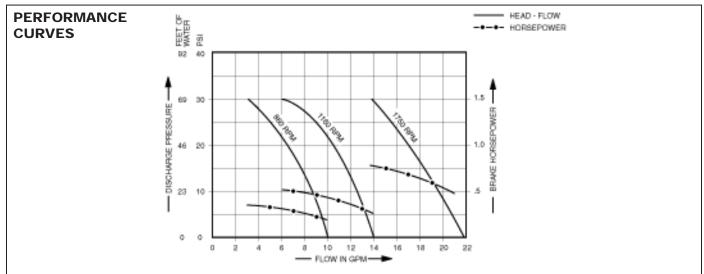
NOTE: Curves show approximate head-flow for new pumps with neoprene impeller pumping water. Capacities should be reduced approximately 10% with nitrile, viton and EPDM impellers.
