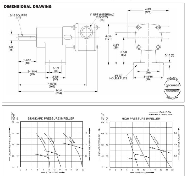
NOTE: Curves show approximate head-flow for new pumps with neoprene impeller pumping water.
