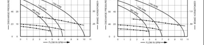
NOTE: Curves show approximate head-flow for new pumps with neoprene impeller pumping water.
