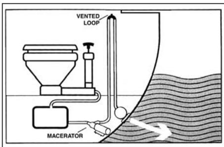
ensure proper priming. Make certain there are no air leaks around the deck plate cap or hose tail. Use minimum 1" (19mm) ID hose for discharge and connect to thru-hull fitting located approximately 4-6 inches above waterline.
