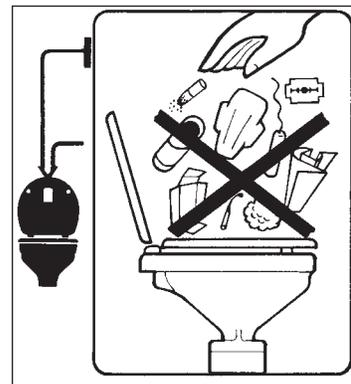
solids such as cigarettes, cigars and chunks of soft fruits or vegetables less than 1" size. It will not pump solid objects like fruit pits, rags, wet strength kitchen towels, tampons or sanitary napkins. The holding tank and pump should be flushed with several gallons of water after each pumpout.
