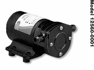
SELECTION OF A COOL, VENTILATED location will generally extend pump motor life. The unit can be mounted in any desired position. It is best to mount so that water dripping from loose port connection will not wet the motor. The pump head may be mounted at 180° increments on the motor to allow change in flow direction.
