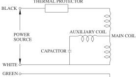
• (W)MD-40R, 40RX, 40RZ, 55R, 70R, 70RZ, and 100R (Single-phase capacitor run motor with thermal protector)
